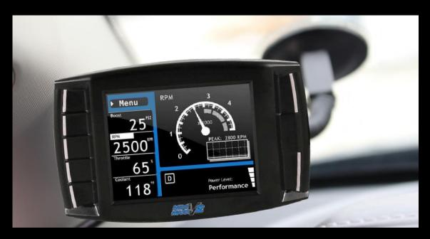
1 After cleaning and drying the windshield, select a safe place to mount the Mini Maxx. Be sure not to obstruct the driver's view when choosing the location.
